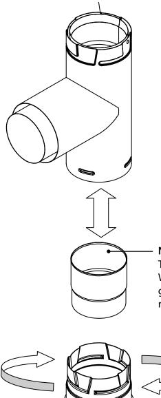
Note: The new PelletVent Pro Tee Cap is a tight fit by design. We recommend using rubber gloves or a strap wrench to remove inner piece.
